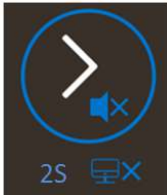
Figure 14: Turn ON/OFF the Panel manually
